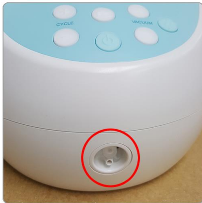
Locate the vacuum nozzle
